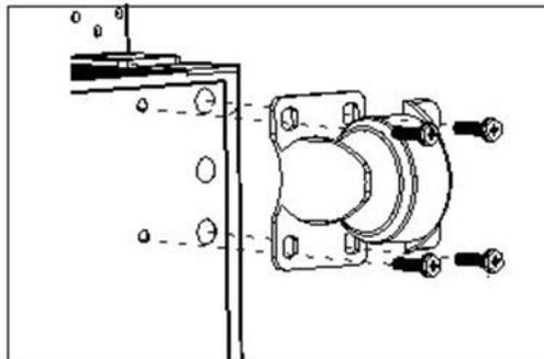
3. The two casters equipped with locks should be installed on the front of the unit
